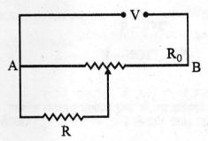
A resistance of R draws current from a potentiometer. The potentiometer wire, AB, has a total resistance of R<sub>o</sub>. A voltage V is supplied to the potentiometer. Derive an expression for the voltage across R when the sliding contact is in the middle of potentiometer wire.
